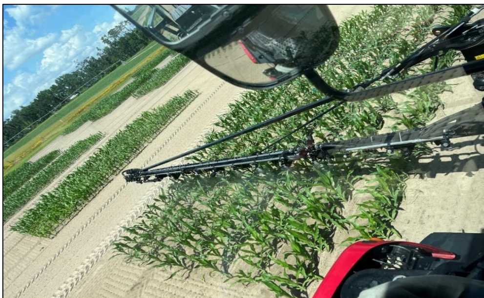
Figure 4. Miller's High Boy 360 y-drop used for liquid side dressing.
